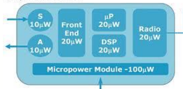
Figure 1 Schematic representation of the major components of a WSN
